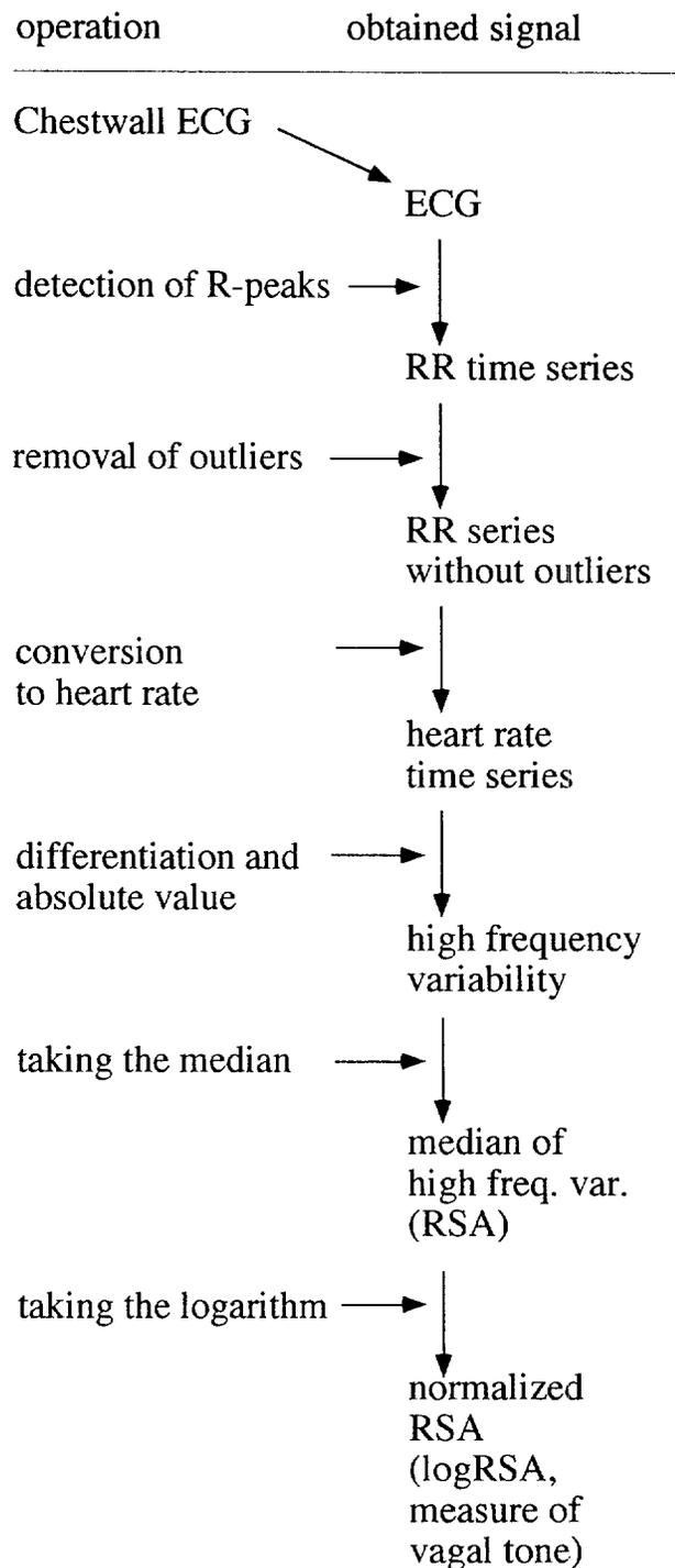
Figure 1. Processing of ECG data to obtain the time-domain measure of cardiac vagal tone (logRSA).
